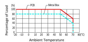
Note: Derate output power by 20% for enclosure (Metal Box) version.
