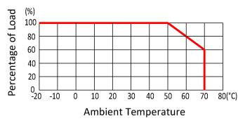
Note: 10 CFM fan cooling is required if total output power is 200W.
